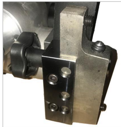
Properly Installed Rail Shoe
